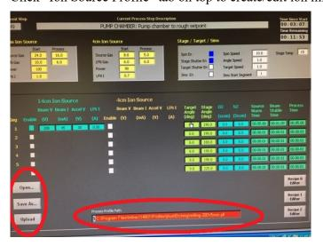
• Click "Open" button and following the screen to load the pre-save recipe. Then click "Upload" button to upload profile to machine for execution. If the current profile does not match the one on the machine, the status bar will turn red and flashing.
