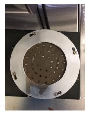
• Following the message in "Current Step Description window", press Process Advance button on the rack to pump the load-lock. Wait until the procedure finish (~10 min). **Do not** interrupt this process.
