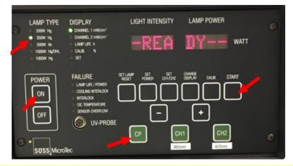
Note: The machine will warn users by beeping if it does not work properly. In case it happens when the lamp is on, turn the main switch to "OFF", leave the system as it is and report to specialist immediately.
